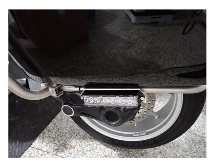
Remove saddlebag by removing the two upper T30 bolts securing the bag to the support.
